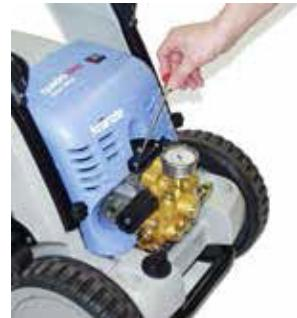
To check the oil level, loosen the oil cover screw and take out the oil dip stick. The oil level must be between the two markings.
