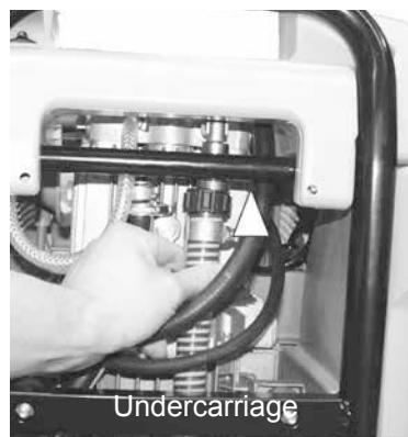
If water is to be sucked from an external container for the high pressure cleaner, the connection hose between the high pressure pump and the water tank must be screwed off and the suction hose must be connected directly to the pump.
