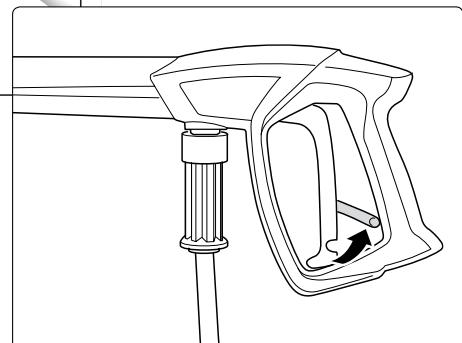
**Apply the safety catch on the spray gun after each use, in order to prevent unintentional spraying!**
