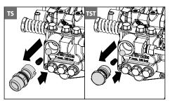
Remove check body and check O-Ring for soiling or damage. Also check seal seat inside pump housing for soiling or damage.
